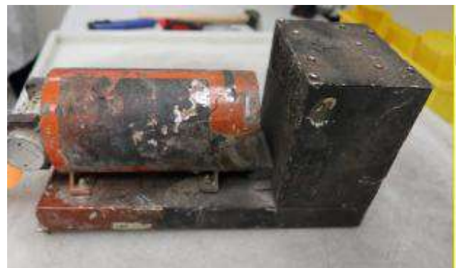
Fig 16 : CVR as recovered from wreckage
