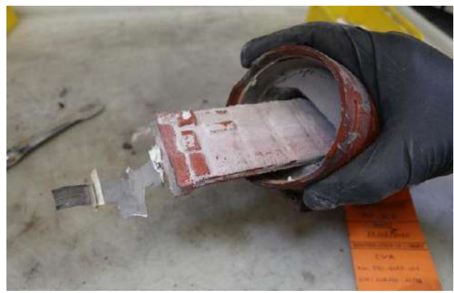
Fig 18 : CVR opening for data recovery
