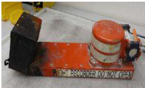
Fig 15 : FDR as recovered from wreckage
