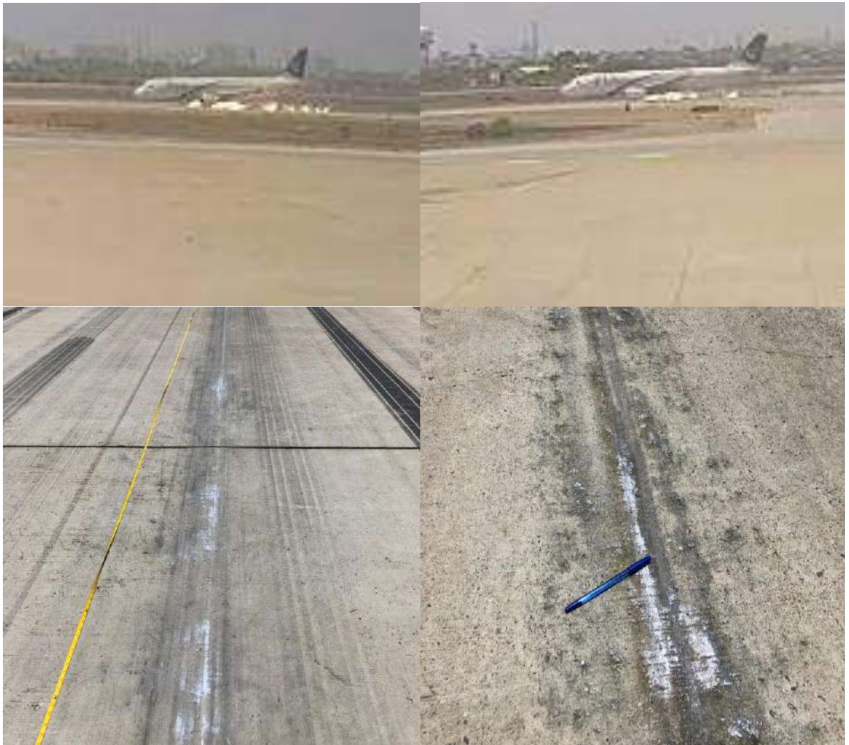
Fig 22 : Screenshots of security / CCTV cameras footages, and marks on runway
