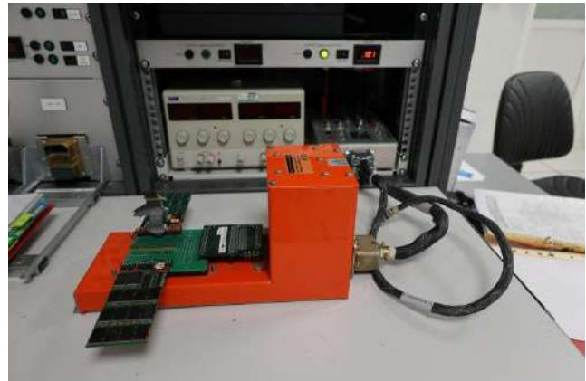
Fig 20 : CVR circuit boards on a golden chassis for readout
