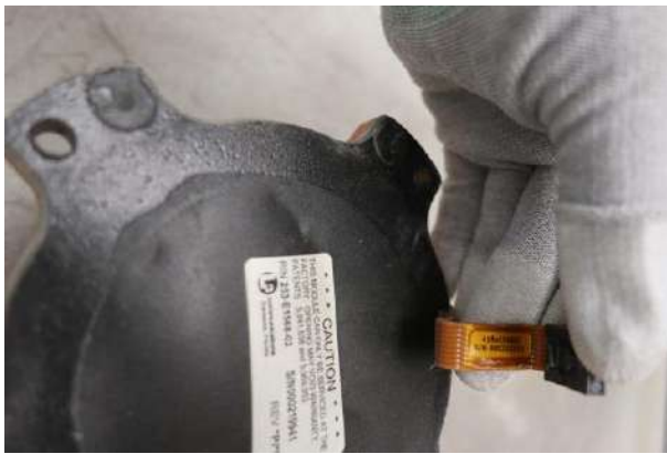
Fig 17 : FDR opening for data recovery
