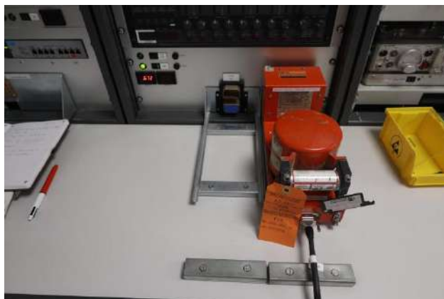
Fig 19 : FDR protected module on a golden chassis for readout
